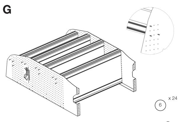
Fasten the aluminium extrusions to the shelf end panels with supplied screws 6 again only half way.
