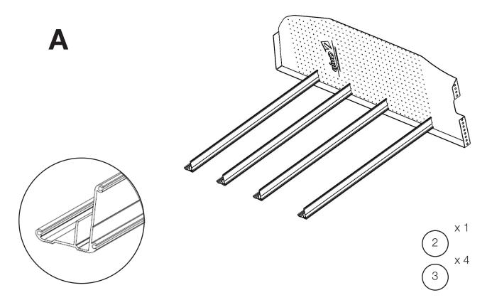
Lay 4 x aluminium extrusions (3) and 1 x shelving end panel (2) on a flat surface as shown
