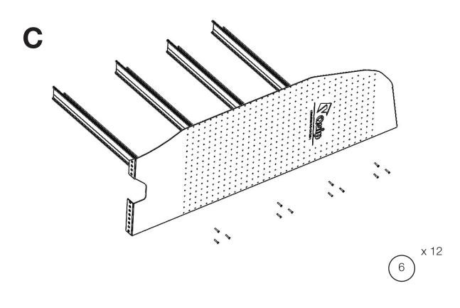
Fasten the aluminium extrusions to the shelf end panel with supplied screws 6 ensuring they are no more than half way in at this stage.
