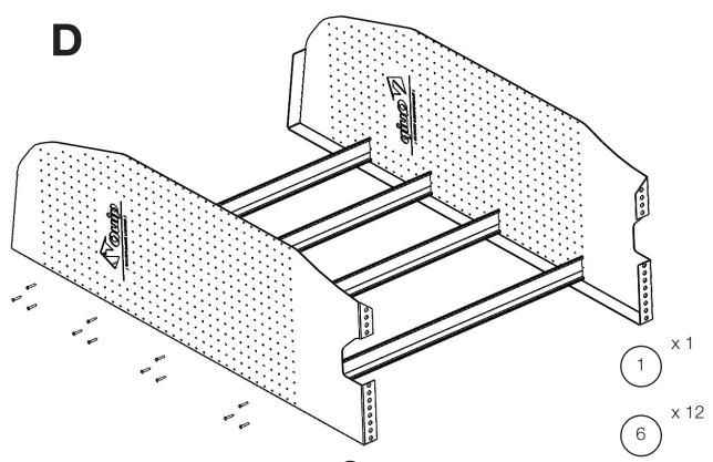
Align the right hand shelf end panel 1 to the other end of the aluminium extrusions (lining up the corresponding holes as shown in step B). Fasten in the same manner as the left hand shelf end panel.
