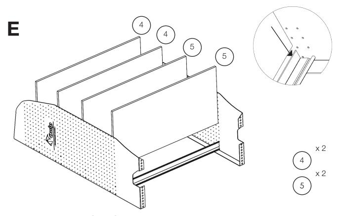
Slide shelf floor panels (4) & (5) into the corresponding extrusions as above.
