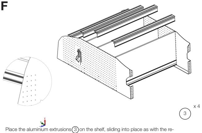
Place the aluminium extrusions (3) on the shelf, sliding into place as with the reverse side. The extrusion guide holes will match up with the corresponding ones on shelf end panel (1)
